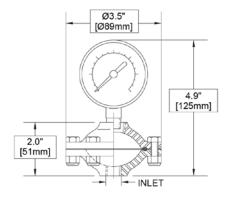
Housing: 316L Stainless Steel Alloy 20 <u>Diaphragm:</u> EPDM PTFE Viton Inlet Size: Up to 0.50"
