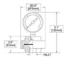
Housing: CPVC PVC Polypropylene PVDF <u>Diaphragm:</u> EPDM PTFE Viton
